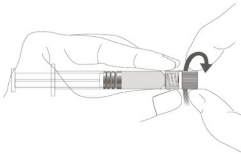
**Step 2:** To attach the needle to the syringe, gently twist the needle clockwise into the syringe until slight resistance is felt.
